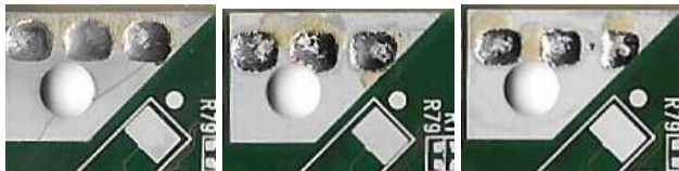
Figure 20a: Solder spread: as plated tin (E) with low SMAP
