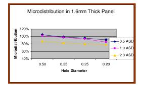
Figure 2 – Microdistribution for 1.6mm Thick Panel
