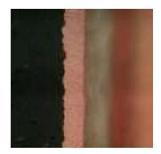
1000x Figure 7 - Cross section of 0.2mmThrough Hole in 1.6 mm Panel Plated at 1.0 ASD
