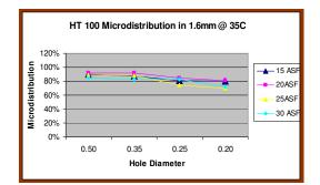
Figure 11 – Microdistribution for 1.6mm Thick Panel Plated 35°C
