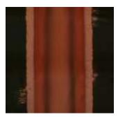
500x Figure 6 - Cross section of 0.2mmThrough Hole in 3.2mm Panel Plated at 0.5 ASD
