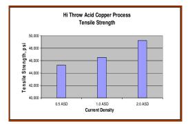
Figure 8 - Tensile Strength versus Current Density
