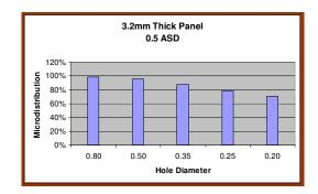
Figure 3 – Microdistribution for 3.2 mm Thick Panel
