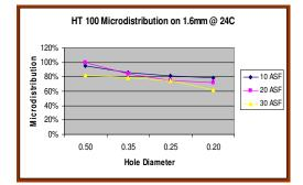
Figure 10 – Microdistribution for 1.6mm Thick Panel Plated 24°C
